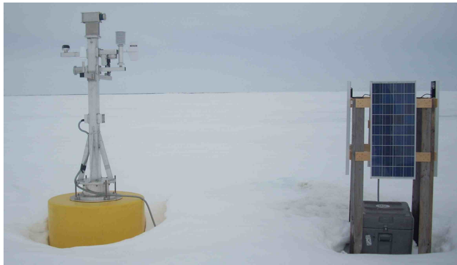
Fig. 6. Photograph of the O-buoy, solar panel array, and lead-acid battery box as deployed during the test phase. During future deployments the solar panels and lead acid packs will be part of the main O-buoy.
