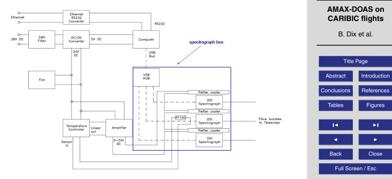
Fig. 5. Block diagram of the electrical connections within the DOAS container instrument.
