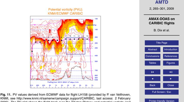
KNMI, see http://www.knmi.nl/samenw/campaign\_support/CARIBIC, last access: 2 February 2009). The PV plot shows the flight track over the Tibetan Plateau and potential vorticity (red contours) with values between 1 and 5 PVU shaded from yellow to red. The blue box indicates elevated PV values in the troposphere, probably caused by a dissolved tropopause fold.
