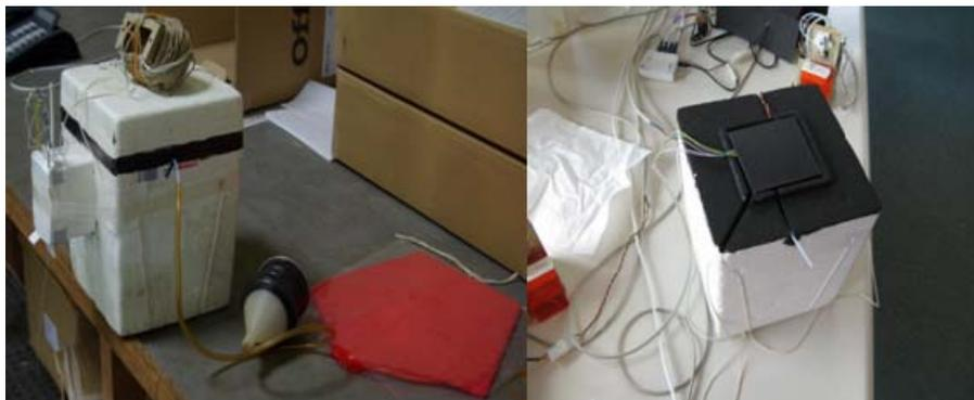
**Fig. 1.** The outside of the NO<sub>2</sub> sonde. On the right side a picture is shown of the inside of the NO<sub>2</sub> sonde, which is painted black so ambient light is absorbed. On the left side a ready-to-use NO<sub>2</sub> sonde.
