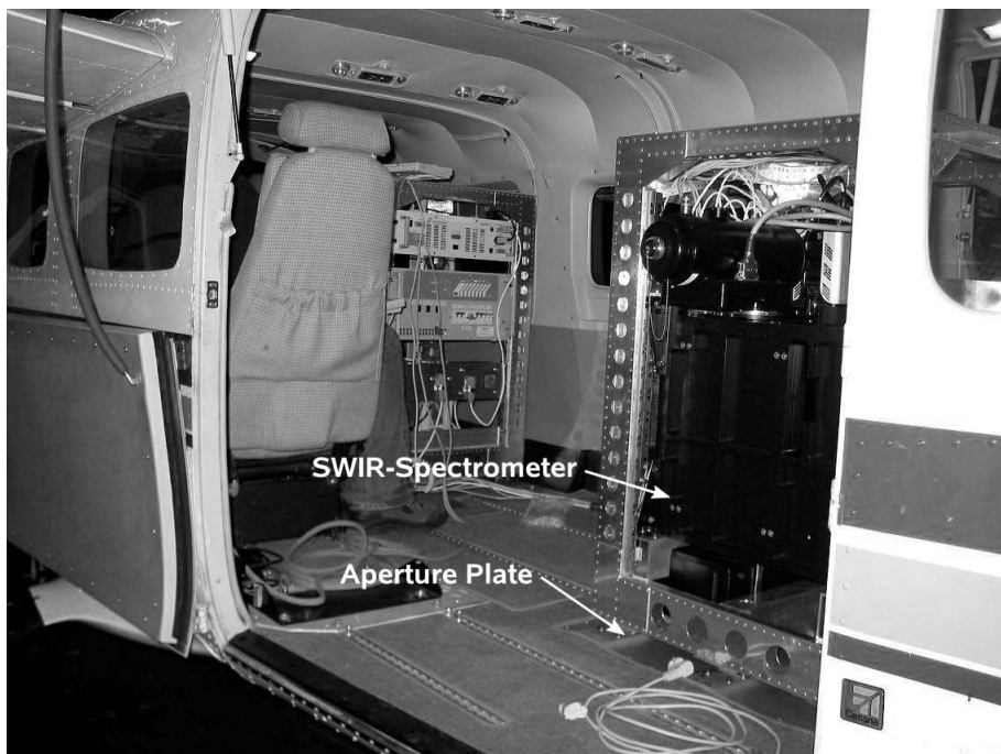
Fig. 4. The MAMAP spectrometer rack mounted on the aperture-plate (front) carrying the optics and the spectrometer systems and the MAMAP auxiliary rack (back) carrying the controllers, power converters and the buffer battery (both racks mounted on the RWE Cessna caravan aircraft).
