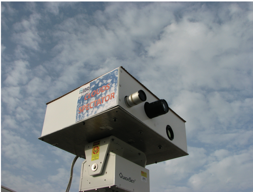
Fig. 1. CLOUDS SPECTATOR measurement assembly. It enables spatial, temporal, and multi spectral sky measurements.
