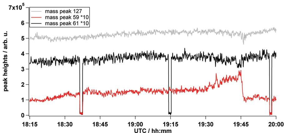
**Fig. 5.** Time series of the ion signals at mass peaks 59 amu ( $^{12}\text{CH}_3^{12}\text{COO}^-$ ), 61 amu ( $^{13}\text{CH}_3^{13}\text{COO}^-$ ) and 127 amu ( $\text{I}^-$ ) for part of the flight on 9 July 2008. Mass peaks 59 and 61 amu are multiplied by a factor of 10. Three instrumental background determinations are shown, at about 18:37 UTC and 19:55 UTC (BCU-mode), and at 19:15 UTC (noLLS-mode). See text for more details.
