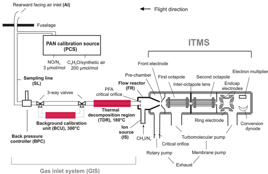
**Fig. 1.** Experimental set-up of the FASTPEX instrument as deployed on the DLR Falcon during the POLARCAT-GRACE campaign 2008. The main components of FASTPEX are a gas inlet system (GIS), a PAN calibration source (PCS), a tubular flow reactor (FR), an ion source (IS) and an ion trap mass spectrometer (ITMS). For more details see text.
