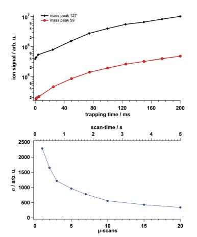
Fig. 2. Ion signals at mass peaks 59 and 127 amu versus the trapping time (upper panel). The lower panel shows the standard deviation at instrumental background conditions (BCU-mode) versus the number of micro-scans (trapping time: 100 ms). The corresponding scan-time is plotted on the top axis.
