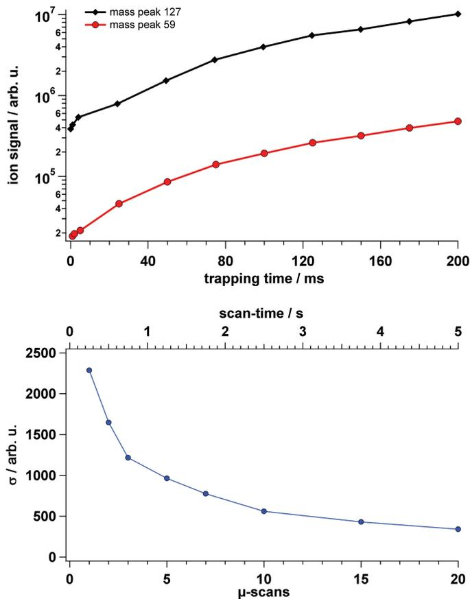
**Fig. 2.** Ion signals at mass peaks 59 and 127 amu versus the trapping time (upper panel). The lower panel shows the standard deviation at instrumental background conditions (BCU-mode) versus the number of micro-scans (trapping time: 100 ms). The corresponding scan-time is plotted on the top axis.
