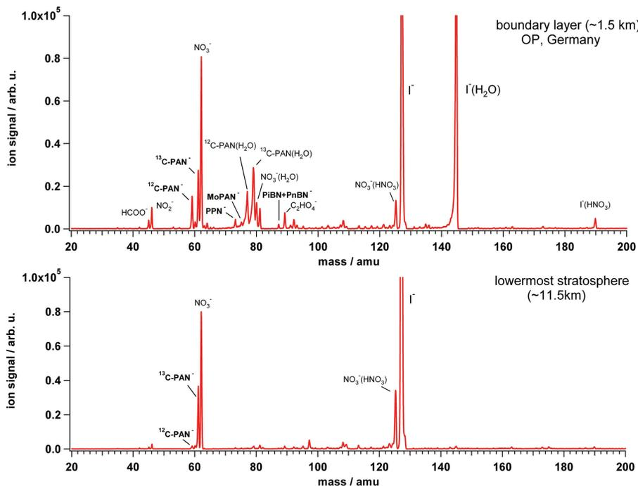
**Fig. 4.** Mass spectra obtained in the polluted boundary layer (BL) over Southern Germany (upper panel) and in the lowermost Arctic stratosphere (lower panel). The high humidity in the BL is reflected in the abundance of hydrated ions whereas the spectrum obtained in the lowermost stratosphere shows almost no hydrated forms. For more details see text.
