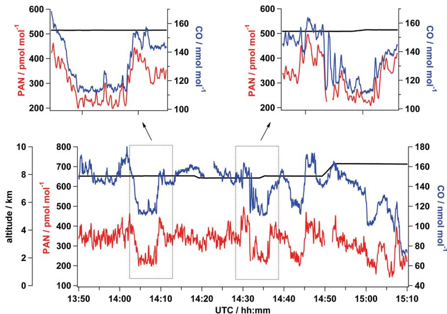
**Fig. 7.** Time series of PAN (2 s) and CO (1 s) for part of the flight on 7 July (13:50–15:10 UTC). An aged Canadian biomass burning plume was intercepted several times at slightly different altitudes, as indicated by elevated PAN and CO concentrations ( $\text{PAN} > 300 \text{ pmol mol}^{-1}$ ,  $\text{CO} > 150 \text{ nmol mol}^{-1}$ ). A blow-up for two parts of the time-series is shown at the top.
