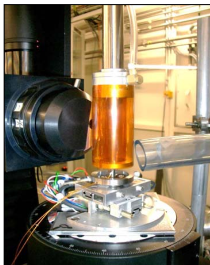
Fig. 1. Experimental setup with the XTM camera microscope on left side. A scheme of the invisible sample holder mounted within the double walled orange Kapton cage mounted on the cryojet nozzle is given on the right side. The Kapton cage can be slid up and down to facilitate sample exchange. The tube from the right pumps away the cold nitrogen exiting at the bottom of the sample holder to prevent water condensation on the goniometer stage.
