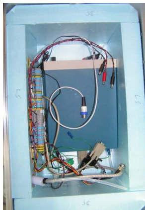
Fig. 2. (a) Schematic of the autonomous ozone monitor system – the blue arrows indicate flow of power; (b) photo of a complete unit installed and measuring; (c) detail of the Teflon inlet system – the metal hoop both holds the inlet tube in place during strong winds, and provides a robust surface against which to knock off any accumulating ice; (d) plan view of the insulated instrument box that housed the ozone monitor (shown) and also the CPU logger enclosure (not shown).
