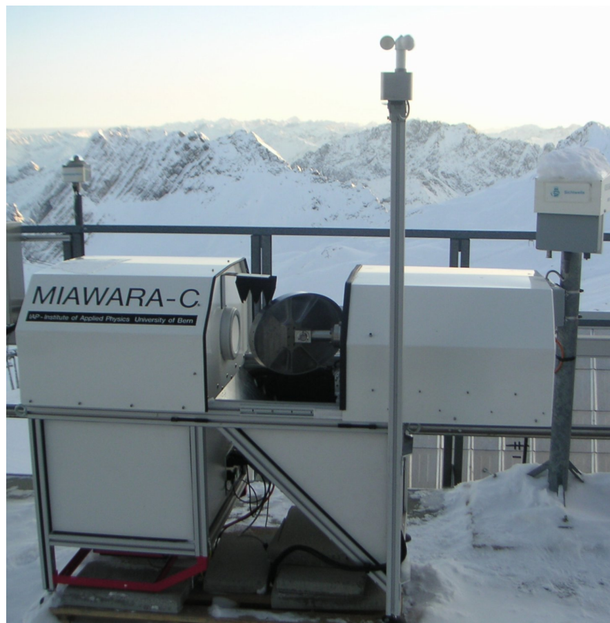
Fig. 2. MIAWARA-C during the ARIS-Campaign on the Zugspitze. The small black absorber above the mirror is used for balancing.
