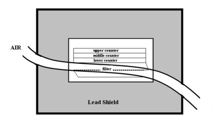
Fig. 1. construction of one-filter detector
