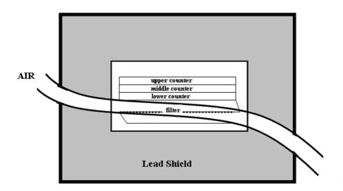
Fig. 1. construction of one-filter detector
