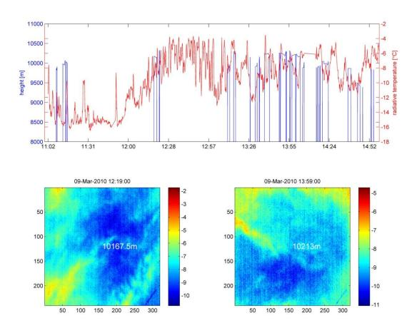
Figure 2 - Cloud base height as extracted by the proposed method during 4 hours on March 9<sup>th</sup>, 2010. The red and blue lines are as in Figure 15. During that time, dense, high cirrus clouds field passed above the sensors. The method produced an average cloud base height of 10,051m with temporal standard deviation of 210m. The two images at the bottom of the figure are examples of specific clouds in that time frame that were extracted by the method.
