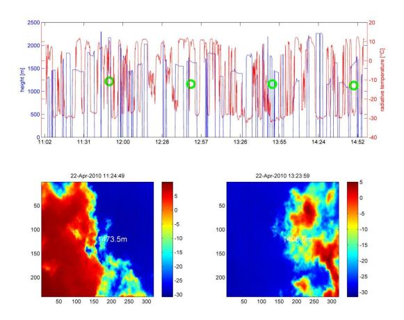
Figure 1 - Cloud base height as extracted by the proposed method during 4 hours on April 22<sup>nd</sup>, 2010. The red line is the radiative temperature of the nadir sky as
