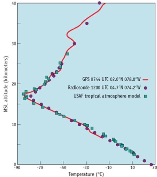
**Fig. 1.** The first radio occultation sounding of earth's atmosphere. The sounding occurred at 07:44 UTC 16 April 1995 over Ecuador. The US Air Force (USAF) mean tropical atmosphere sounding and a nearby radiosonde profile are also shown. Sounding was from GPS/MET and the retrieval was done by Ben Herman at the University of Arizona. A similar version was published by Ware et al. (1996).
