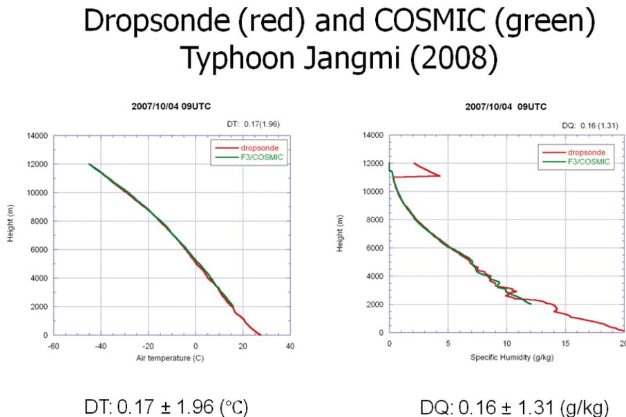
**Fig. 21.** Comparison of FORMOSAT-3/COSMIC atmospheric retrieval profile with high-resolution in-situ dropsonde data. Left panel: temperature (°C). Right panel: Specific humidity (g/kg) (Source: Po-Hsiung Lin, National Taiwan University, 2010).
