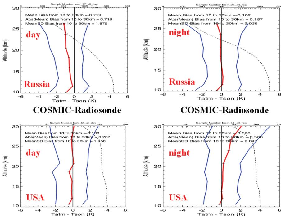
**Fig. 4.** Comparison of two different types of radiosonde (Russian and US) with COSMIC RO observations during the day and night. The red curves are the mean differences. The two blue curves are the standard deviation of the differences. The dashed black line is the number of pairs at each level. The RO soundings, which are not affected by sunlight, reveal biases in the Russian radiosondes during the day and the US radiosondes during the night (He et al., 2009).
