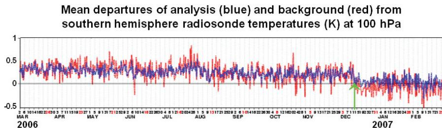
**Fig. 27.** Time series of the mean and standard deviations of the ECMWF background and analysis temperatures at 100 hPa showing a reduction in the bias errors on 12 December 2006 when COSMIC data began to be assimilated (green arrow) (Luntama et al., 2008).
