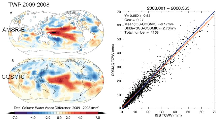
**Fig. 36.** Left: Differences in precipitable water derived from AMSR-E and COSMIC soundings from 2008 to 2009. Warm colors indicate 2009 was wetter than 2008; cool colors indicate 2009 was drier than 2008 (Mears et al., 2010). Right: Correlation of precipitable water in mm estimated from ground-based GPS (IGS TCWV) and COSMIC (COSMIC TCWV) (Ho et al., 2010a).
