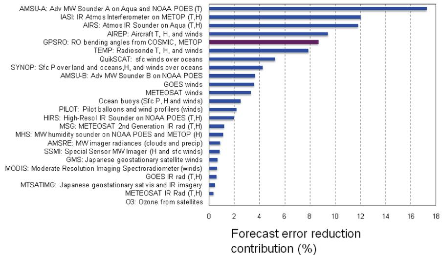
**Fig. 30.** Contribution to the reduction in forecast error (in percent) by all the observing systems used by the ECMWF. RO is the fifth most important observing system in reducing forecast error (Cardinali, 2009a,b).
