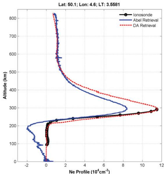
**Fig. 37.** An example of profiles of Abel and data assimilation retrievals of electron density ( $N_e$  in  $10^4 \text{cm}^{-3}$ ) compared to a co-located ionosonde-observed electron density profile (Yue et al., 2011).
