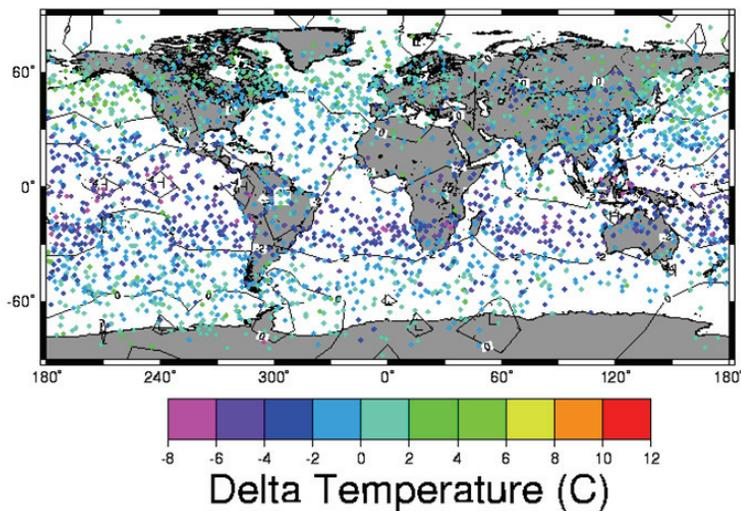
**Fig. 26.** GPS/MET minus NCEP-NCAR reanalysis temperatures ( $^{\circ}\text{C}$ ) at 100 hPa. Note the systematic differences in the equatorial regions between GPS/MET and NCEP. NCEP is significantly warmer than GPS/MET in the equatorial regions and somewhat cooler in middle latitudes (Anthes et al., 2000).
