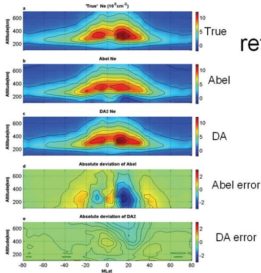
**Fig. 38.** Altitude-latitude cross sections of electron density ( $\text{Ne}$  in  $10^5 \text{ cm}^{-3}$ ) at midday (Local time LT=13). The top panel is the assumed “true” Ne cross section. The second and third panels from the top are the cross sections obtained from the Abel and data assimilation retrievals, respectively. The 4th and 5th panels from the top show cross sections of the errors associated with the Abel and data assimilation retrievals, respectively (Yue et al., 2011).
