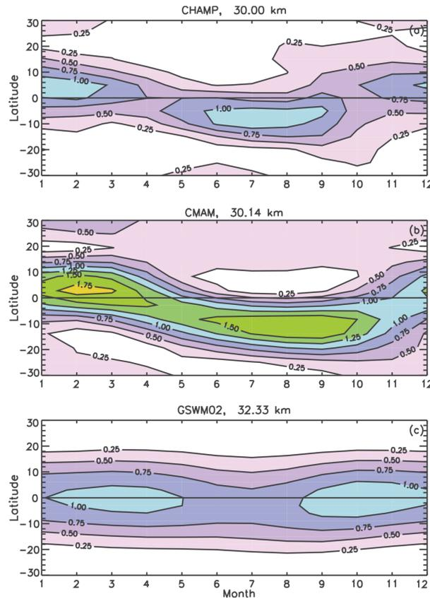
**Fig. 15.** Amplitudes of the diurnal tide near 30 km as a function of latitude and month from the (top) CHAMP RO observations (May 2001–August 2005) and (middle) Canadian Middle Atmosphere Model (CMAM) and (bottom) GSWM02 model simulations. The contour interval is 0.25 K (Zeng et al., 2008).
