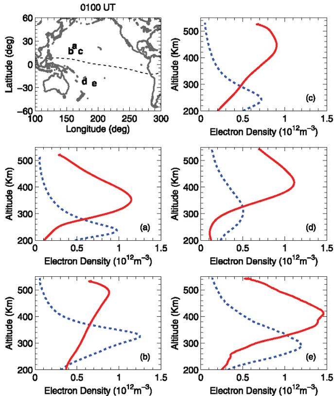
**Fig. 40.** Comparison of vertical electron density profiles from COSMIC on 14 December 2006 (before the geomagnetic storm, dashed blue) and 15 December 2006 (after the storm, solid red). The locations of the electron density profiles are indicated in the map at the top left (Pedatella et al., 2009).
