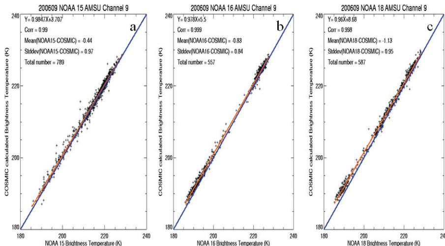
**Fig. 33.** Use of COSMIC data to calibrate AMSU on NOAA satellites. NOAA 15 brightness temperature ( $T_b$ ) vs. COSMIC  $T_b$  (left); NOAA 16  $T_b$  vs. COSMIC  $T_b$  (middle); and NOAA 18  $T_b$  vs. COSMIC  $T_b$  (right). Units of  $T_b$  in K (Ho et al., 2009a).
