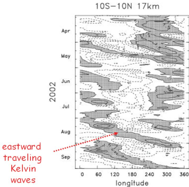
**Fig. 12.** Kelvin wave variability near the equatorial tropopause observed in CHAMP GPS radio occultation measurements. Longitude-time diagrams of zonal wave numbers 1–2 temperature variations over 10° N–10° S during April–September 2002. Contours are 0.5, 1.5, and 2.5 K (Randel and Wu, 2005).
