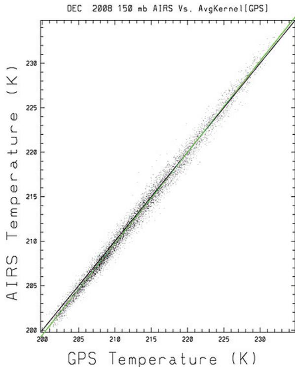
**Fig. 34.** Correlation of AIRS and COSMIC temperatures (K) at 150 hPa for December 2008. AIRS temperatures are slightly lower (higher) than COSMIC temperatures for lower (higher) temperatures (Ho et al., 2010b).
