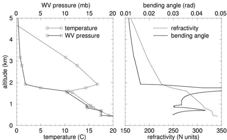
**Fig. 23.** Temperature ( $^{\circ}\text{C}$ ) and water vapor pressure (mb) (left) and corresponding bending angle and refractivity (right) profiles associated with a well-defined ABL. The bending angles reach a sharp maximum at the top of the ABL, which is characterized by large vertical gradients of temperature and water vapor (Sokolovskiy et al., 2007).
