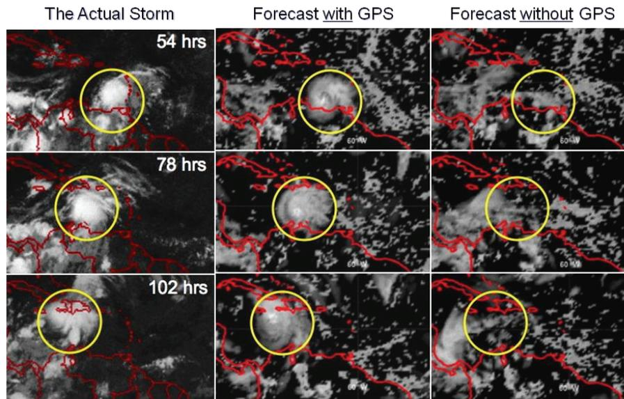
**Fig. 22.** Forecasts of tropical cyclone Ernesto (2006) using the NCAR WRF (Weather Research and Forecast) model. Images on the left are actual satellite photos of the event. Images on the right were generated from a forecast made without RO data, while the images in the center are from a forecast that assimilated 15 RO profiles. The elapsed time since the beginning of the forecast is shown on the left-hand images – in this case, 54, 78 and 102 h (Liu et al., 2011).
