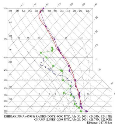
**Fig. 20.** CHAMP soundings compared to two radiosondes in Typhoon Toraji (2001). The CHAMP temperature and water vapor profiles are computed from the observed refractivity and a 1D-VAR algorithm (Anthes et al., 2003).
