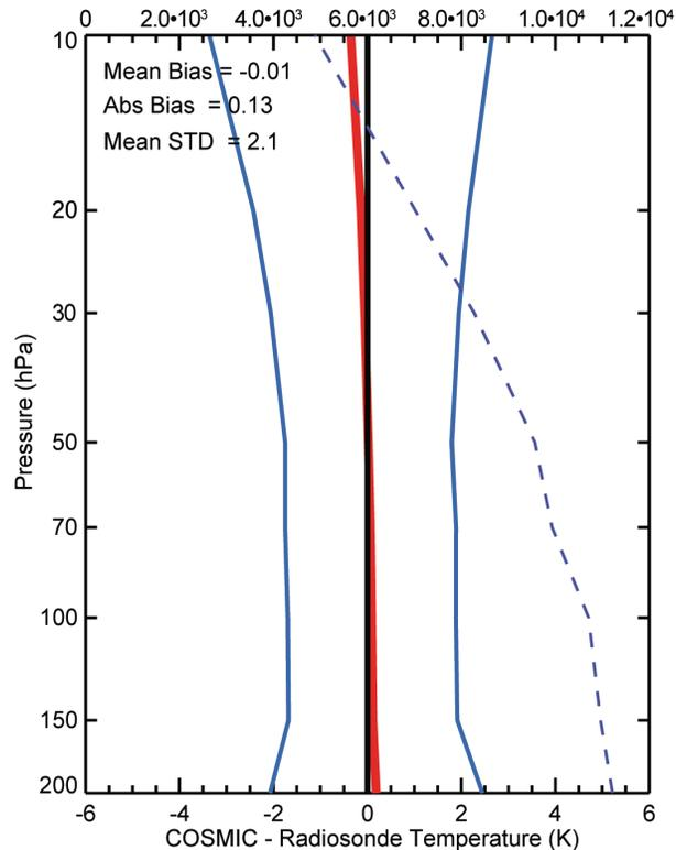
**Fig. 6.** Statistics of a comparison between COSMIC and high-resolution accurate radiosondes between 10 and 200 hPa. This comparison shows that the accuracy of RO observations in this regions is 0.13 K or higher. The number of pairs in the comparisons is shown by the blue dashed line and the scale at the top. The mean difference is shown by the red line and the standard deviation of the differences by the solid blue lines. (Ho et al., 2010a).
