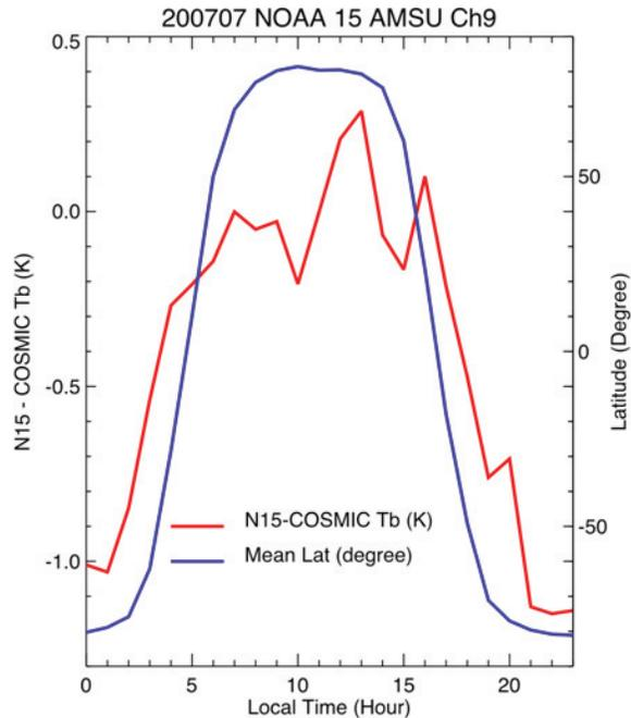
**Fig. 35.** NOAA-15 AMSU brightness temperatures ( $T_b$ ) minus COSMIC  $T_b$  as a function of local time. Since the RO brightness temperatures are not affected by temperature variations of the satellites, the differences in  $T_b$  between the COSMIC and the NOAA-15 data are an indication of local-time biases in the NOAA-15 data. As shown in this figure, these differences follow a pattern similar to the mean latitude vs. local time (Ho et al., 2009b).
