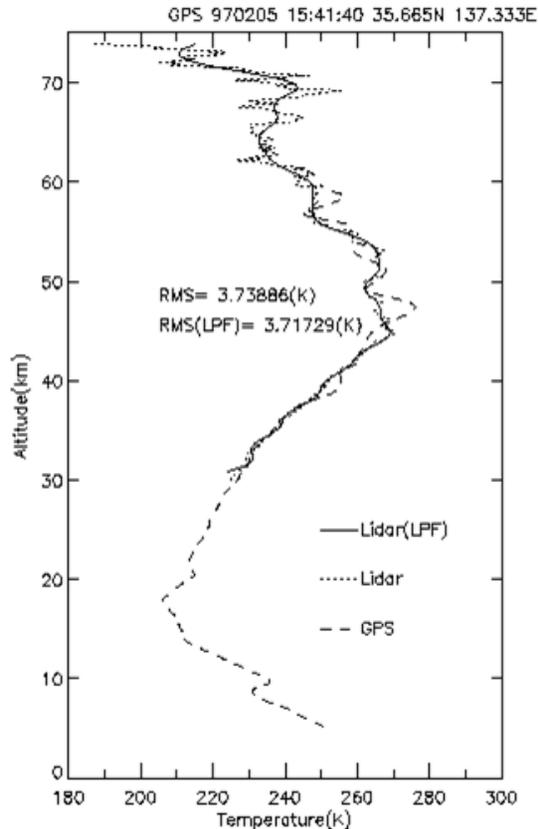
**Fig. 10.** Comparison of temperature profiles between GPS/MET data (dashed lines) at 15:41 UTC 5 February 1997 at 35.7° N, 137.3° E and Rayleigh lidar data (dotted line) between 15:08 and 16:26 UTC at 36.1° N, 140.1° E (Tsuda et al., 2000).
