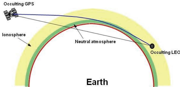
**Fig. 2.** Geometry of RO limb scanning technique. As the Low-Earth Orbiting (LEO) satellite carrying a GPS receiver rises or sets behind earth, a series of scans of earth's atmosphere is obtained. The bending of the radio waves is determined through precise measurements of the phase changes and used to compute bending angle, refractivity and other products at high vertical resolution.
