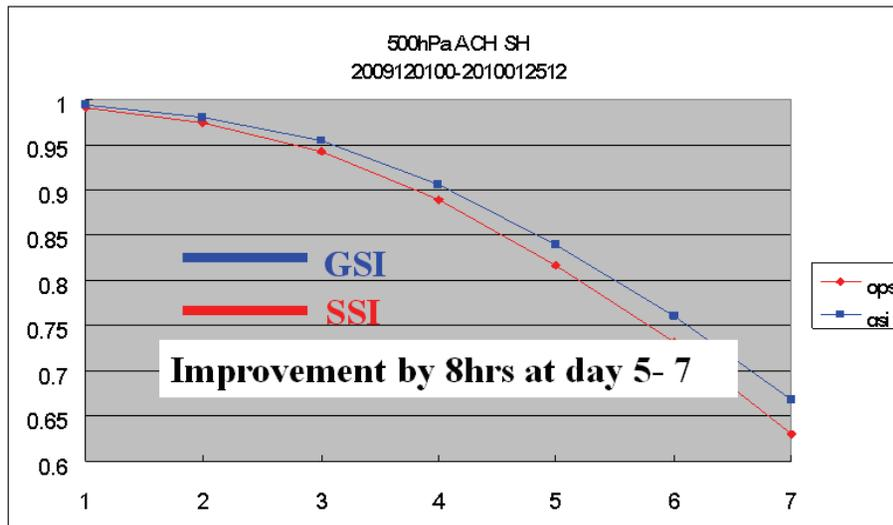
**Fig. 29.** Effect on forecast 500-hPa height anomaly correlation at the Central Weather Bureau (CWB), Taiwan during December 2009–January 2010 after COSMIC data were introduced. The significant, positive impact is produced by the improvement of RO data assimilation between SSI and GSI (Dr. Chin-Tzu Fong, Central Weather Bureau, personal communication, 2010).
