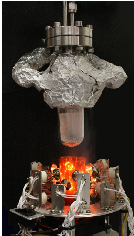
Fig. 2. Photo showing the sublimation vessel with a loaded ice sample and the infrared source. The cooling jacket starts just above the ice sample and a cold air stream is fed in from both sides. The infrared source consists of 18 bulbs mounted on a holder, and the red foil visible in the central part. During the sublimation of the ice sample the infrared source is moved upwards, hence the section with sample is surrounded by the bulbs.
