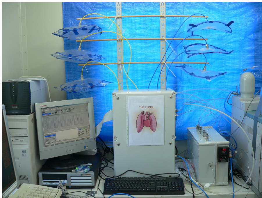
Fig. 3. “Lung-GC system” set-up in mobile laboratory trailer. The “Lung” is in the centre of the picture and corresponds to the shaded box in Fig. 1. The set of bags on the left (Cluster B) are being filled while those on the right (Cluster A) are being evacuated. Ribs on the bags help to keep them flat. To the right of The Lung is the Valco stream selection valve (mounted inside the box) and further to the right the GC can just be seen. To the left of the Lung is the GC control and acquisition PC and the LabVIEW ® PC controlling the entire process.
