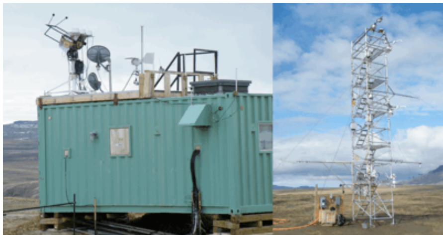
Fig. 4. SAFIRE rooftop is instrumented with tracker-mounted radiometers (left). At 10.5 m height, the flux tower is equipped with four radiometers (right).
