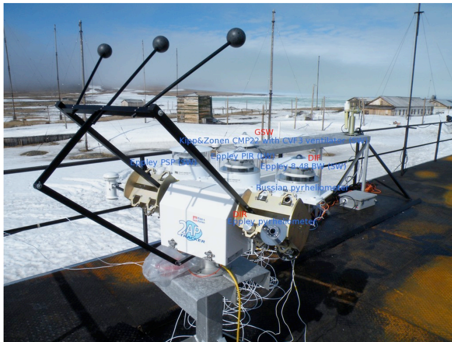
Fig. 2. Solar tracker mounted surface radiation sensors in Tiksi, Russia. Shortwave measurements are made by GSW (global shortwave), DIR (direct), and DIF (diffuse) sensors.
