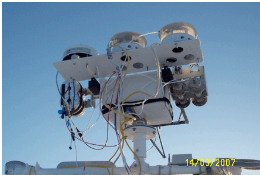
Fig. 6. Example solar tracker and its circuit box wrapped in the arctic rated blanket.
