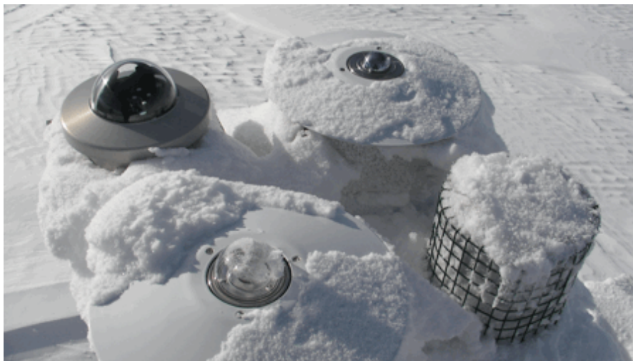
Fig. 7. SPN-1 radiometer (upper left), ventilated Eppley PSP radiometer (lower left) and ventilated Eppley PIR pyrgeometer (upper right). A thin layer of frost on the PSP's dome is clearly visible.
