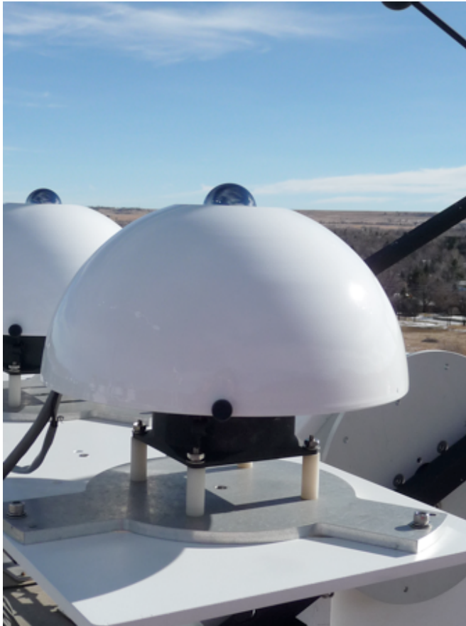
Fig. 9. Example radiometer with arctic rated ventilator.
