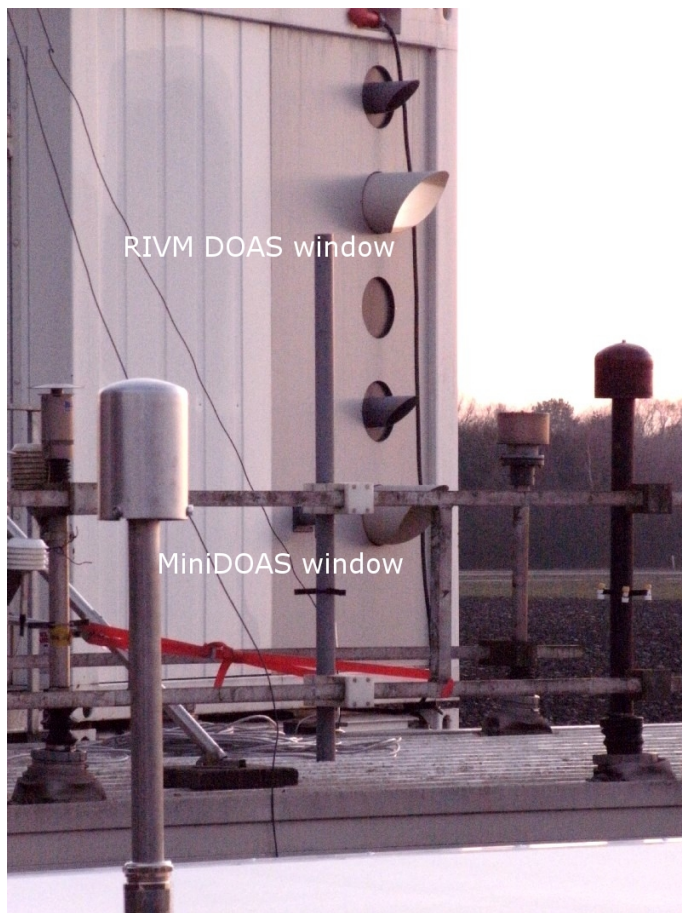
Fig. 12. Photo of measurement cabin with the two windows, of the RIVM DOAS (upper window, with light emerging) and the miniDOAS (lower window, partly hidden by a metal rail). The light of the lamps are directed directly over the inlet of the AMOR instrument inside the LML measurement cabin.
