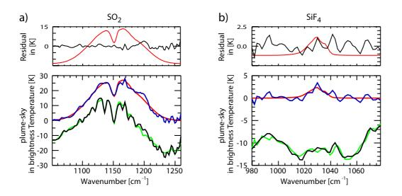
**Fig. 3.** Spectral regions where  $SO_2$  (a) and  $SiF_4$  (b) are retrieved at  $4 \text{ cm}^{-1}$  resolution. Lower plots: The difference of a plume spectrum and a reference-sky spectrum are shown in black and the corresponding fits in green. The same is plotted above for the spectra (blue) and fits (red) when all other fit parameters (continuum radiation and interference gases) are removed. Above: the residuals of the fits for each retrieval window.
