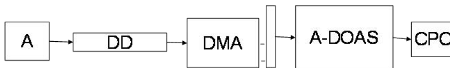
Fig. 3. A flow diagram of experimental setup used to measure the optical properties of a monodisperse PSL sample with the AE-DOAS. A = atomizer, DD = diffusion dryer, DMA = differential mobility analyzer, AE-DOAS = aerosol extinction differential optical absorption spectrometer, which is shown in detail in Fig. 1, and CPC = condensation particle counter. Additional instrument details are given in the experimental section.
