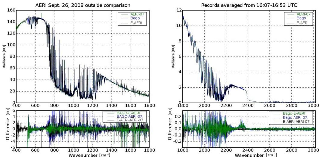
**Fig. 4.** Radiance measurements during two outside side-by-side tests performed at UW. Top panels display measured radiance ( $\text{RU} = \text{mW}/(\text{m}^2 \text{sr cm}^{-1})$ ) with residuals in the bottom panels.
