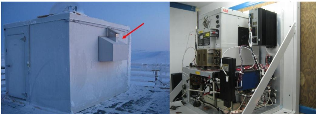
**Fig. 1.** Exterior (left panel, red arrow) and interior (right panel) views of the E-AERI installed on the roof of the PEARL Ridge Lab using the thru-wall configuration. Left panel: the hatch is closed during precipitation events (Photo: Stephane Lantagne). Right panel: the back-end of the E-AERI instrument with its internal protective enclosure removed, showing the MR-300 series interferometer housing and electronics (Photo: Zen Mariani).
