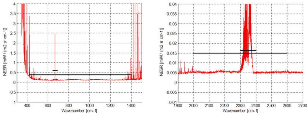
**Fig. 2.** NESR test for the MCT (Left panel) and InSb (right panel) detectors performed in Eureka. The solid black line indicates the specified requirement for the NESR test. The elevated black line indicates the spectral region where the NESR is expected to increase due to CO<sub>2</sub> in the instrument.
