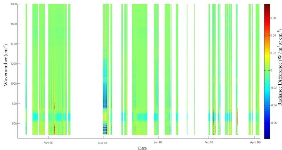
**Fig. 8.** Hourly-averaged coincident radiance difference measurements (P-AERI–E-AERI) from 22 October 2008–5 April 2009. Only the longwave radiances are shown for clarity. White spaces correspond to periods with no measurement overlap due to precipitation or instrument maintenance.
