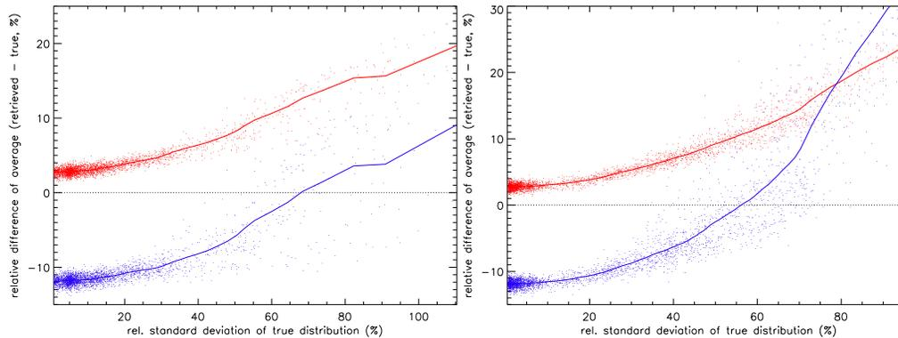
**Fig. 4.** Differences of retrieved and “true” zonal means (relative to the latter) versus local natural variability in terms of standard deviation for CO (left) and H<sub>2</sub>O (right). Red: linear averages, blue: logarithmic averages. Data points reflect individual latitude/altitude boxes. Results are shown for maximum likelihood ln(vmr)-retrieval simulations with a signal to noise ratio of 2.
