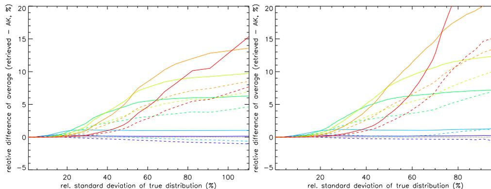
**Fig. 7.** Differences between the mean values and the mean “true” atmospheric state after application of the averaging kernel to the latter for CO (left) and H<sub>2</sub>O (right). Solid: linear averages, dashed: logarithmic averages. Results are shown for maximum a posteriori  $\ln(\text{vmr})$ -retrieval simulations with SNRs of 10 (dark blue), 5 (light blue), 2 (dark green), 1.43 (light green), 1.0 (orange), and 0.5 (red).
