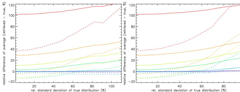
**Fig. 5.** Differences of retrieved and “true” zonal means (relative to the latter) versus local natural variability in terms of standard deviation for the CO (left) and H<sub>2</sub>O (right). Solid: linear averages, dashed: logarithmic averages. Results are shown for maximum likelihood ln(vmr)-retrieval simulations with signal to noise ratios of 10 (dark blue), 5 (light blue), 2 (dark green), 1.43 (light green), 1.0 (orange), and 0.5 (red).
