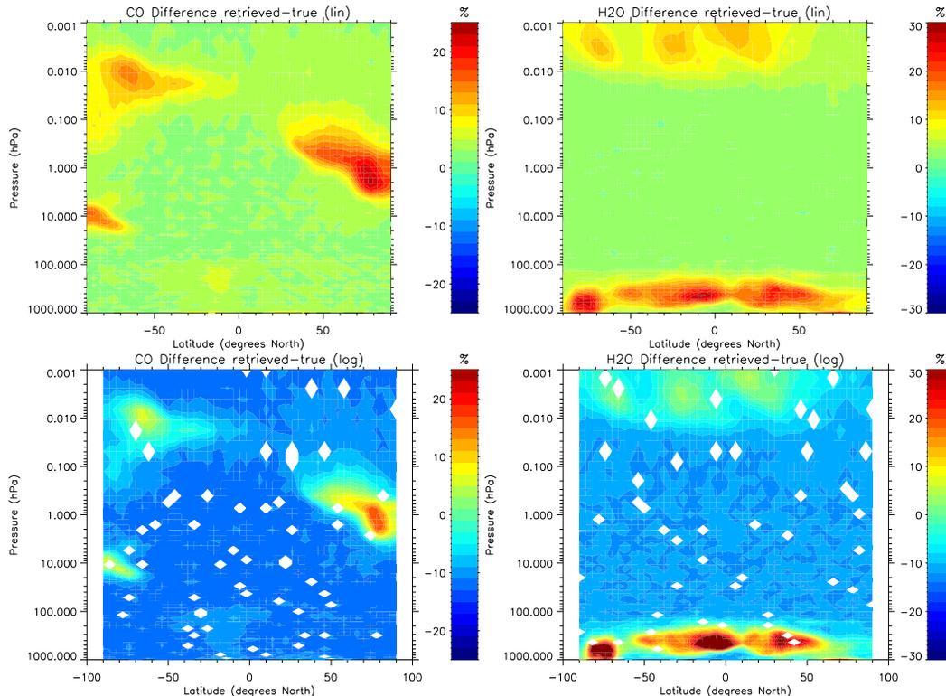
**Fig. 3.** Zonal mean differences of retrieved and “true” distributions (relative to the latter) for CO (left) and H<sub>2</sub>O (right). Top: linear averages, bottom: logarithmic averages. Results are shown for maximum likelihood ln(vmr)-retrieval simulations with a signal to noise ratio of 2. White regions in the lower panels reflect unreasonable results (“zero” averages, see text for further explanations).
