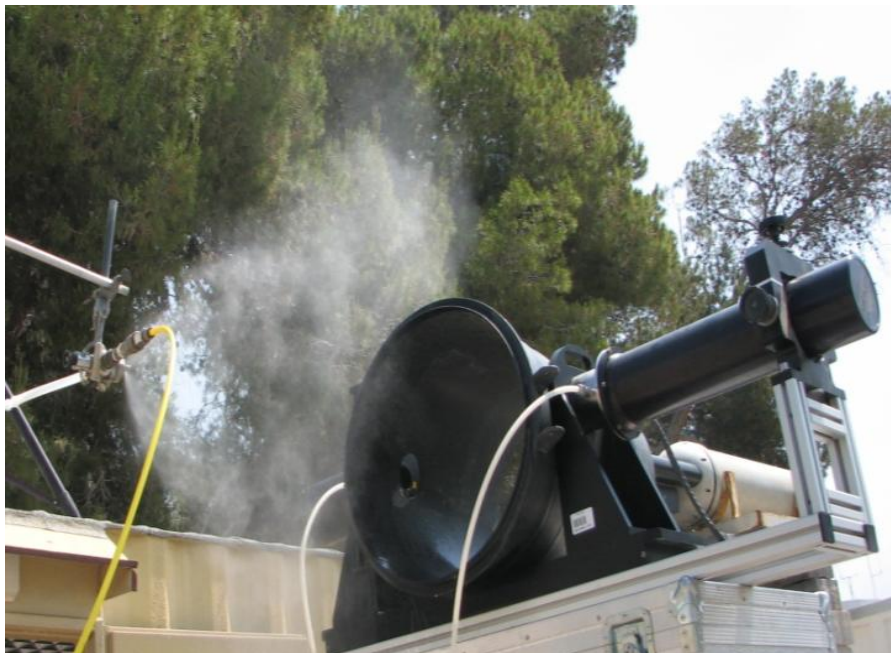
Fig. 20. A controlled experimental setup for validation of the proposed methodology. An artificial cloud was sprayed via an air-atomizing nozzle and entered the field of view of an accurate particle sizing device (Spraytec). A calibrated spectro-radiometer and a thermal imager were positioned below the passing cloud (not shown), pointing to the zenith.
