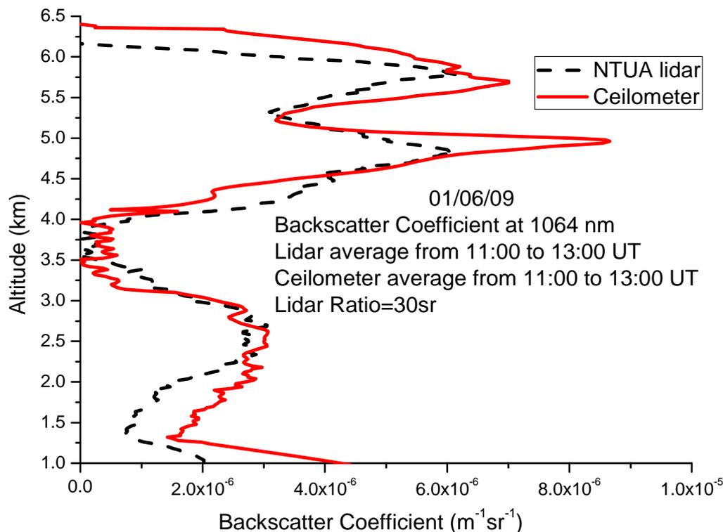
**Figure. 10.** Average vertical profiles of the aerosol backscatter coefficient obtained by the Vaisala ceilometer (11:00–13:00 UTC) and the NTUA Raman lidar system (11:00–13:00 UTC) on 1 June 2009.
