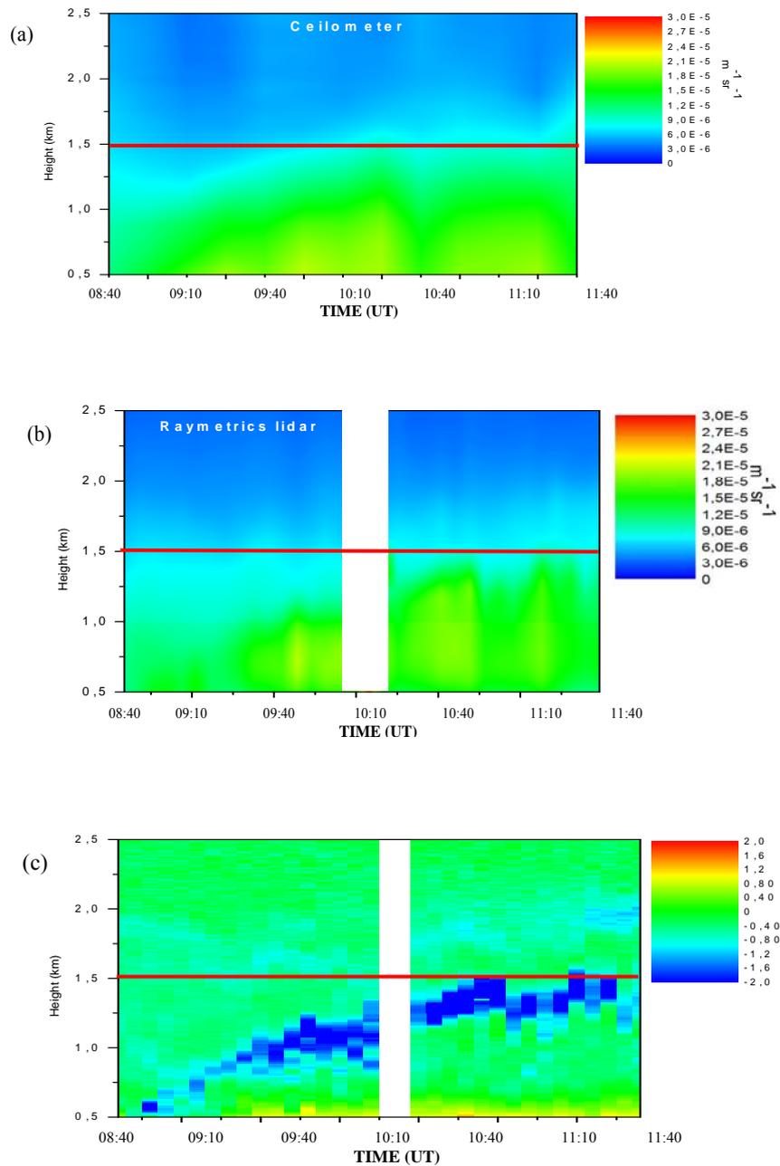
**Fig. 2.** Aerosol backscatter coefficient (in  $\text{m}^{-1} \text{sr}^{-1}$ ) obtained (a) by the ceilometer and (b) the Raymetrics lidar. (c) The first derivative of the logarithm of the range-corrected lidar signal (in A.U.) obtained by the Raymetrics system. All curves are valid from 08:40 to 11:35 UTC on 27 November 2008. Red lines represent mean PBL height around 12:00 UTC.
