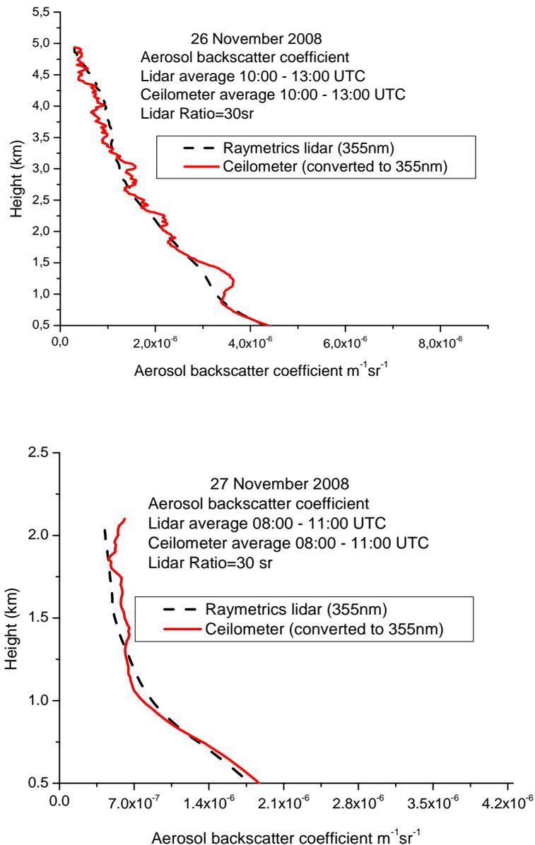
**Fig. 4.** Comparison of the aerosol backscatter coefficient profiles obtained by the Vaisala ceilometer and the Raymetrics lidar (a) on 26 November and (b) on 27 November 2008.
