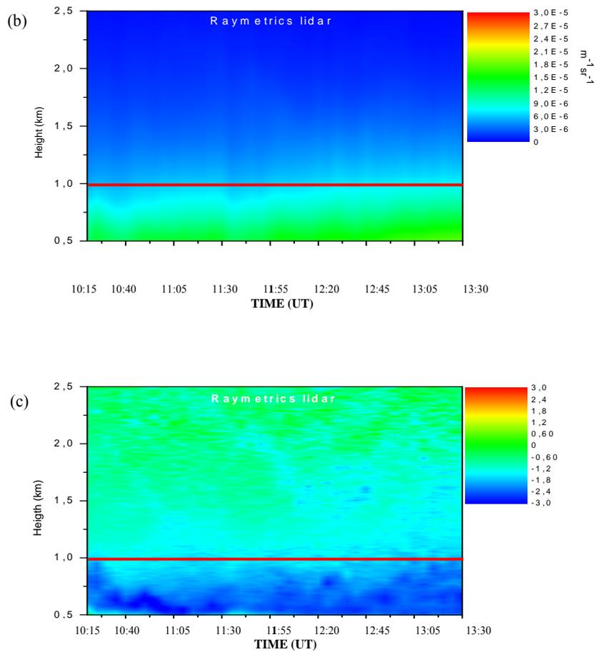
**Fig. 1.** Aerosol backscatter coefficient (in  $\text{m}^{-1}\text{sr}^{-1}$ ) obtained (a) by the ceilometer and (b) the Raymetrics lidar. (c) The first derivative of the logarithm of the range-corrected lidar signal (in A.U.) obtained by the Raymetrics system. All curves are valid from 10:15 to 13:45 UTC on 26 November 2008. Red lines represent mean PBL height around 12:00 UTC.
