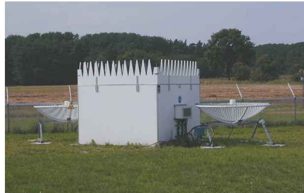
Fig. 1. Bi-static RASS antenna set up. \alpha scattering angle, h measuring height, D distance between electromagnetic transmit and receiving antennas.
