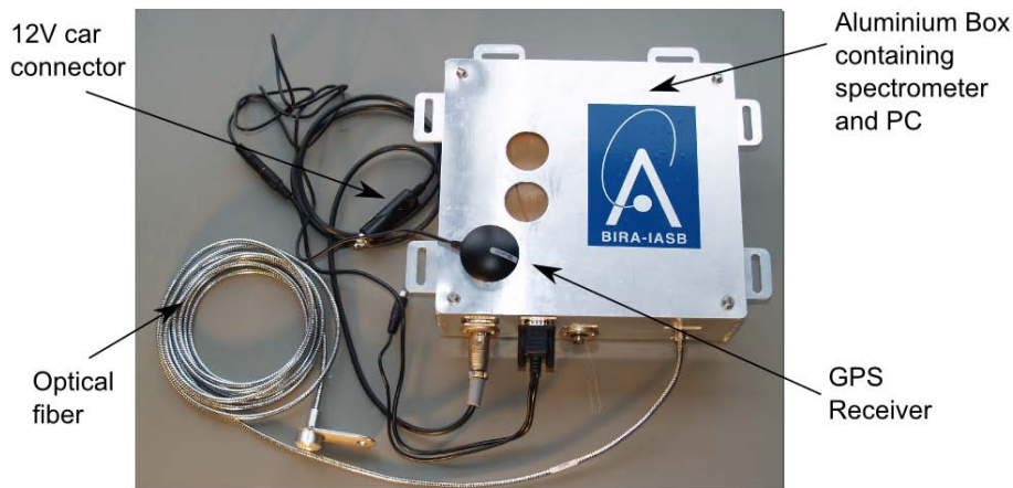
Fig. 2. The ULMDOAS instrument. Inside the box are a compact uv-vis spectrometer and a PC-104. Light is collected directly by the optical fiber and a GPS is used to geolocalize the measurements. The whole system is powered with 12v.
