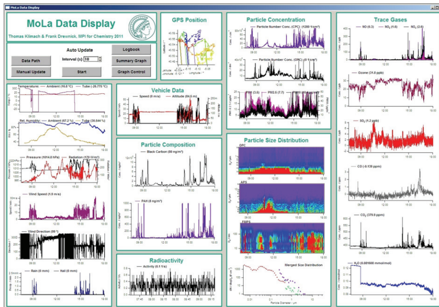
Fig. 5. Data live display tool of the mobile laboratory showing time series and current measurement data of all parameters (except AMS data and webcam image) on a single screen. Graph control, summary graphs and logbook functions are activated by buttons on the top left.
