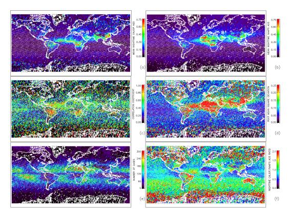
Fig. 4. For 2007 at 1° × 1° global resolution, (a) mean nighttime CALIOP 0.532 μm AOD, (b) corresponding mean nighttime NAAPS 0.550 µm AOD (see text), (c) correlation coefficient between the two datasets for all points inclusive, (d) root mean square deviation between the two, (e) number of corresponding cases per grid bin and (f) the ratio of corresponding mean nighttime CALIOP/NAAPS AOD. Points with no data coincide with a white pixel color that is no represented on the color bar.
