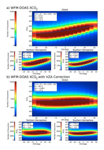
**Fig. 7.** WFM-DOAS  $XCO_2$  v2.1 VZA dependency before (a) and after (b) the scan-angle-bias correction. (a) 2-D-histogram of WFMDv2.1  $XCO_2$  versus the VZA using all data between 2003 and 2009. The blue curve is a quadratic fit. (b) As (a) but after the bias correction.
