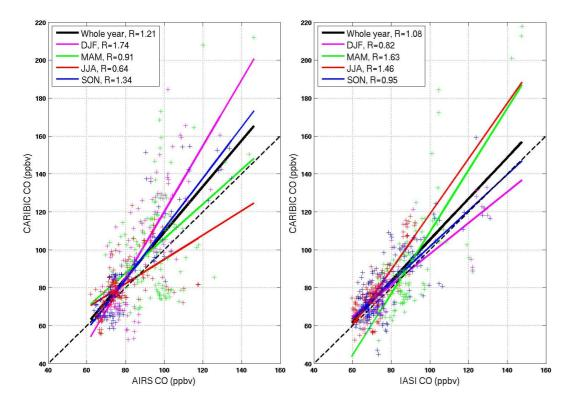
**Fig. 5.** Scatter plots of  $1^{\circ} \times 1^{\circ}$  averaged CARIBIC and AIRS (left panel) and IASI (right panel) CO. The coloured lines represent the linear regression between the data for each season (pink: December-January-February, green: March-April-May, red: June-July-August, blue: September-October-November) and the black line for all seasons. The black dashed line gives the 1:1 line.
