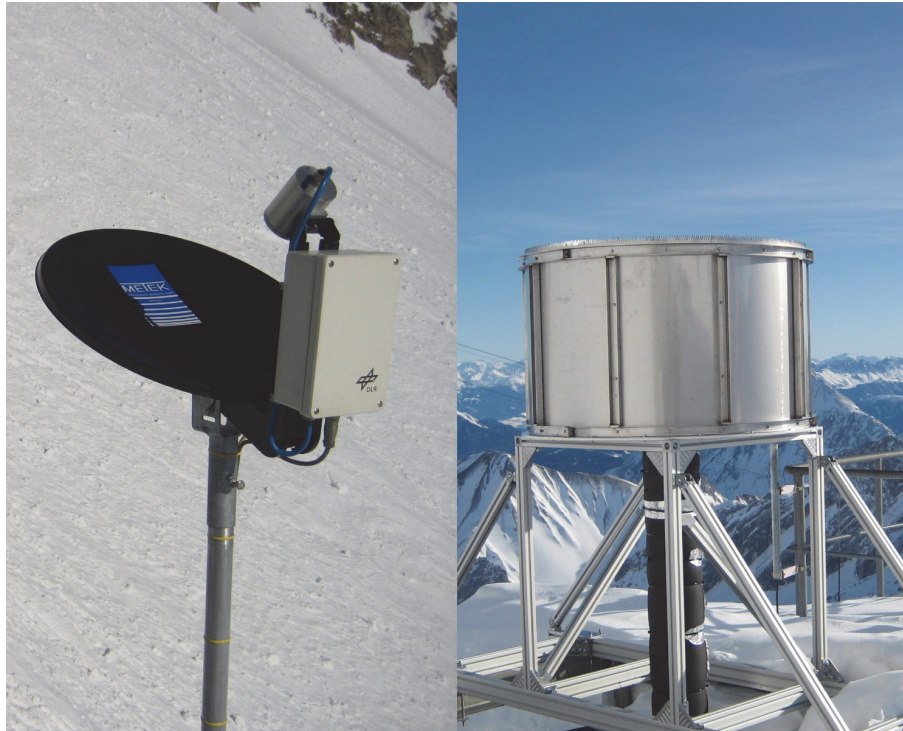
Fig. 1. Micro Rain Radar 2 (MRR) (left) and MIRA35 cloud radar (right) at the UFS Schneefenerhaus.
