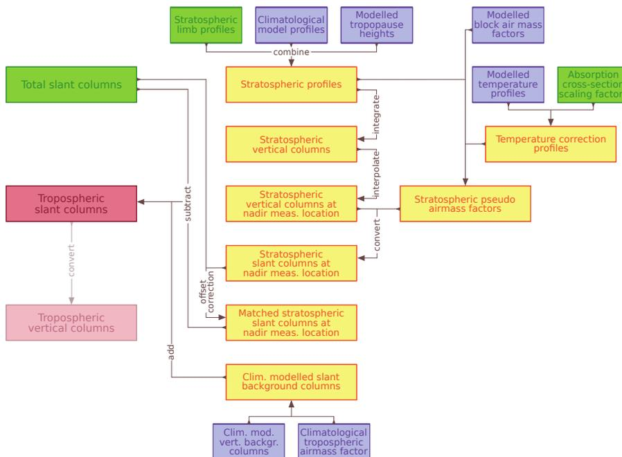
**Fig. 1.** Data flow of calculating tropospheric NO<sub>2</sub> columns from SCIAMACHY measurements. Measured and modelled quantities are shown in green and purple, respectively, while intermediate results are marked in yellow. Conversion of SCD<sub>trop</sub> to VCD<sub>trop</sub> involves calculation of tropospheric air mass factors, the discussion of which is beyond the scope of this study.
