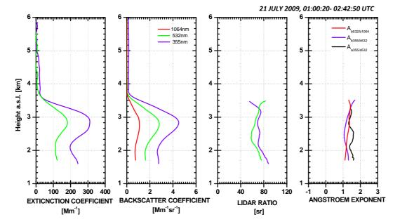
**Fig. 4.** Vertical profiles of the aerosol optical parameters (extinction, backscatter, lidar ratio, Ångström exponent) retrieved by the EOLE Raman lidar measurements on 21 July 2009 (01:20–02:42 UTC).
