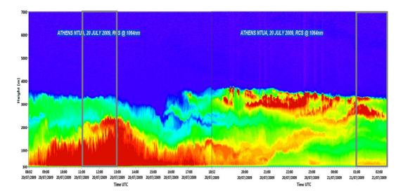
**Fig. 3.** Temporal evolution of the range-corrected lidar signal (RCS) obtained over Athens at 1064 nm, between 08:02 UTC (20 July 2009) and 02:42 UTC (21 July 2009). The grey panels refer to the aircraft flight periods.
