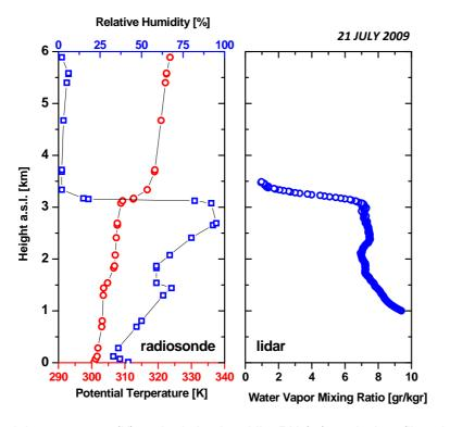
**Fig. 6.** Potential temperature (K) and relative humidity-RH (%) vertical profiles obtained from radiosonde data on 21 July 2009 (00:00 UTC) (left panel) and water vapor mixing ratio derived from the EOLE Raman lidar measurements on 21 July 2009 (01:20–02:42 UTC).
