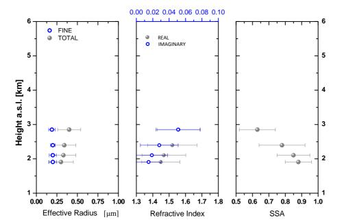
**Fig. 5.** Retrieved aerosol effective radius  $(r_{\text{eff}})$ , refractive index (m) and single scattering albedo  $(\omega)$  based on the aerosol optical properties derived by the EOLE Raman lidar on 21 July 2009.
