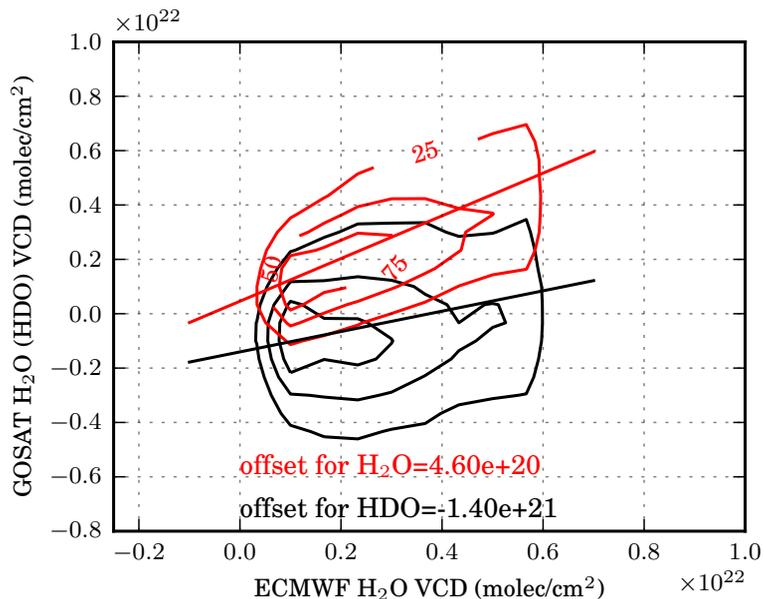
**Fig. 2.** Frequency distribution and linear fit of retrievals and ECMWF estimates over very dry regions (mostly Antarctica coincidences chosen here). Contour lines show 25, 50 and 75 percentile distributions. Small offset errors in both HDO and H<sub>2</sub>O column estimates can be observed, and fitted offsets are used in the subsequent bias correction.
