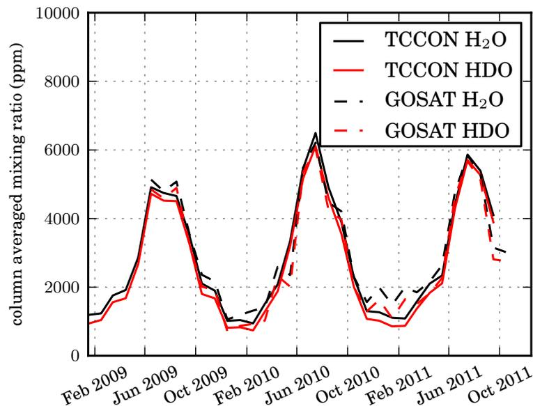
**Fig. 4.** Comparison of monthly HDO and H<sub>2</sub>O column amounts over the Lamont (Oklahoma) TCCON station (GOSAT coincidences within  $\pm 3^\circ$  latitude and longitude).
