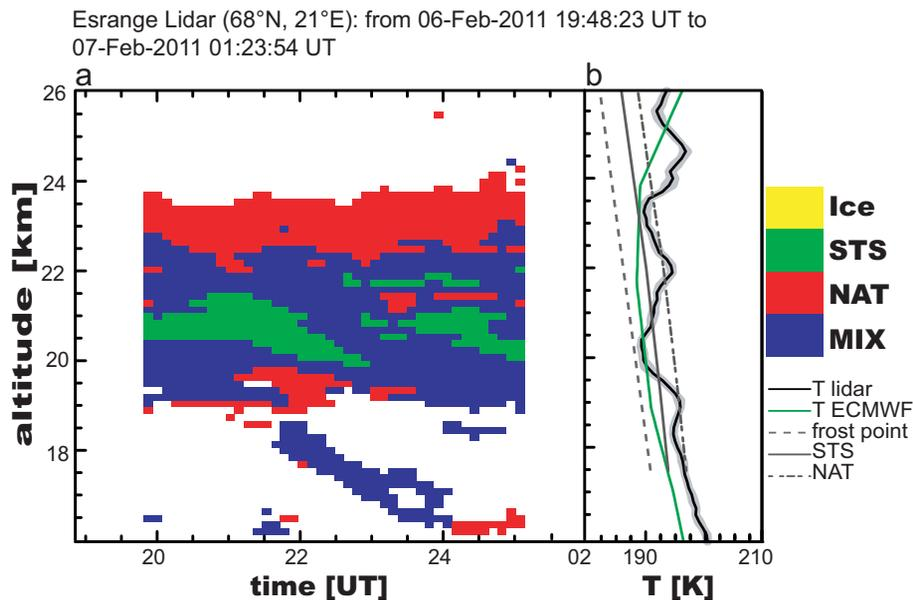
**Fig. 5.** (a) Development of a PSC above Esrangle on 6 February 2011 between 19:48 and 01:23 UT. (b) Temperature profile (black) and the error in the temperature (grey area) derived over the entire measurement period in comparison to ECMWF from 00:00 UT on 7 February 2011. Grey lines indicate the formation and existing temperatures for PSC of type: ice (dashed), STS (solid), and NAT (intermittent).
