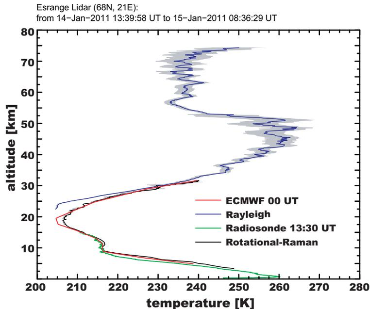
**Fig. 4.** Temperature profile between 5 and 75 km measured at Esrangle between 13:39 UT on 14 January 2011 and 08:36 UT on 15 January 2011. Profile were obtained using the integration technique (blue) and the rotational-Raman technique (black). The grey shaded area shows the error range. For comparison the temperature profiles measured with radiosonde (green) and given by the ECMWF re-analysis (red) are shown as well.
