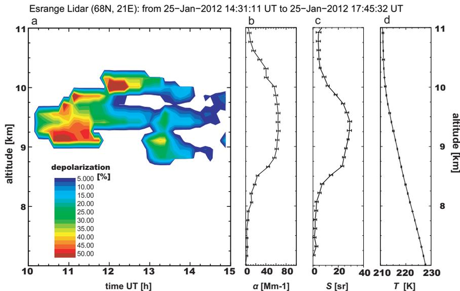
**Fig. 6.** (a) Development of a cirrus cloud above Esrange between 14:31 and 17:45 UT on 25 January 2012 in terms of the particle depolarization ratio and profiles of the extinction coefficient  $\alpha$  (b), the lidar ratio  $S$  (c), and temperature  $T$  (d).
