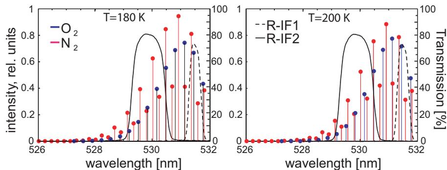
**Fig. 2.** The line-by-line pure rotational-Raman spectrum (only anti-Stokes) of  $O_2$  (blue) and  $N_2$  (red) calculated for  $T = 180$  K (left) and  $T = 200$  K (right) and the transmission curve of the two interference filters (R-IF1 with a central wavelength line (CWL) at 531.55 nm and R-IF2 with a CWL at 529.35 nm) produced by Barr Associates, Inc.
