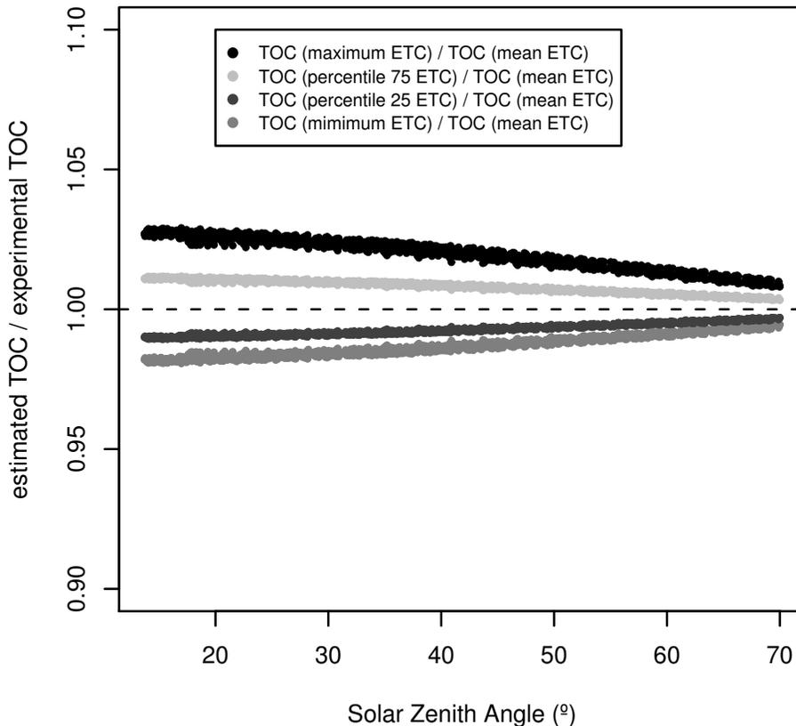
**Fig. 2.** The ratio of the estimated and the experimental total ozone column as a function of the solar zenith angle for the 30 selected cloud-free half-days. The experimental total ozone data have been derived using the mean ETC value while the estimated data using the maximum, minimum, percentile 75 and 25 ETC values.
