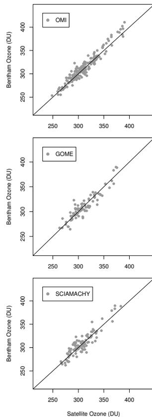
**Fig. 4.** Correlation between satellite and ground-based TOC data gathered over the Granada for the period between April 2005 and May 2006. (top) OMI versus Bentham. (middle) GOME versus Bentham. (bottom) SCIAMACHY versus Bentham. The solid line represents the unit slope with which the data almost agree. DU, Dobson units.
