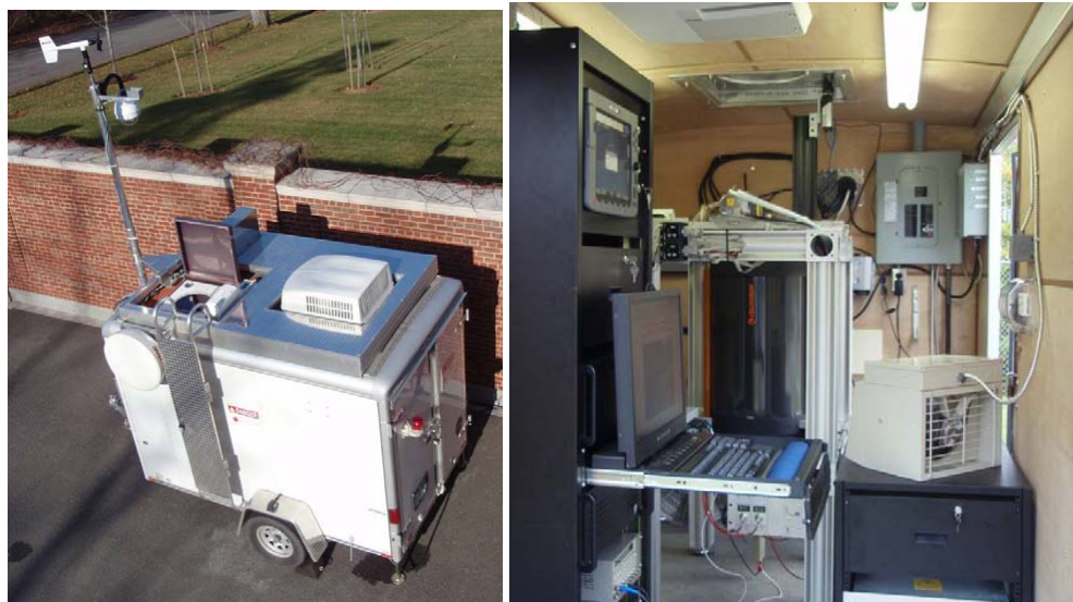
Fig. 1. (a) A picture showing the outside of the portable, autonomous aerosol lidar system. Note the location of the hatch assembly, radar and meteorological tower and (b) a picture of the inside of the trailer showing the basic layout of the lidar optical bench and rack locations.
