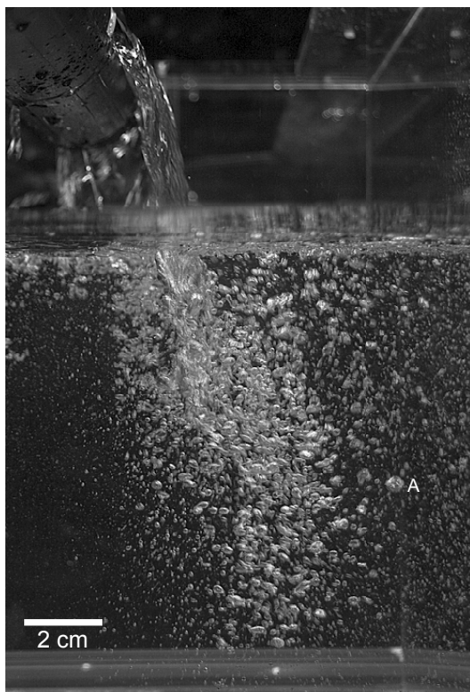
Fig. 3. Side view of plunging sheet and bubble plume. Bubble A is approximately 2.2 mm in radius, demonstrating the presence of bubbles larger than the Hinze scale. The free-fall distance between the exit slot of the waterfall and the water surface is approximately 10 cm, but appears shorter due to the angle at which the photograph was taken. The width of the plunging sheet is approximately 20 cm.
