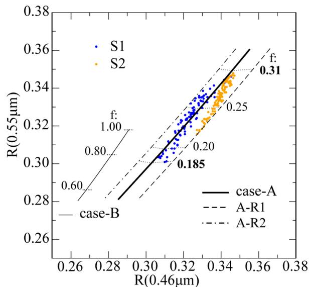
**Fig. 3.** Simulated values of the reflectance  $[R(\lambda p)]$  for aerosol models with size parameter ( $f$ ) and the refractive indices ( $m$ ) (refer to Table 2) in a two-channel diagram at wavelengths of 0.46 and 0.55  $\mu\text{m}$ . The blue and yellow dot symbols denote the satellite data S1 and S2 in Fig. 2, respectively, observed on 21 September of 2005 by Aqua/MODIS.
