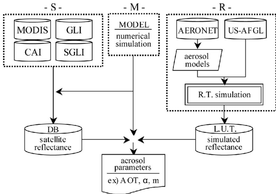
**Fig. 1.** A block diagram for satellite-based aerosol retrieval.
