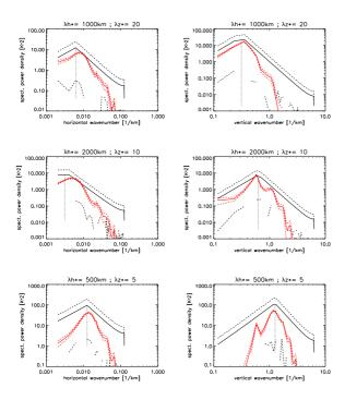
**Fig. 1.** Comparison of (red) S3D and (black) 1D Fourier transform spectra for (left colum) horizontal and (right colum) vertical coordinates. The solid lines give the average spectrum, dashed lines for the FT
