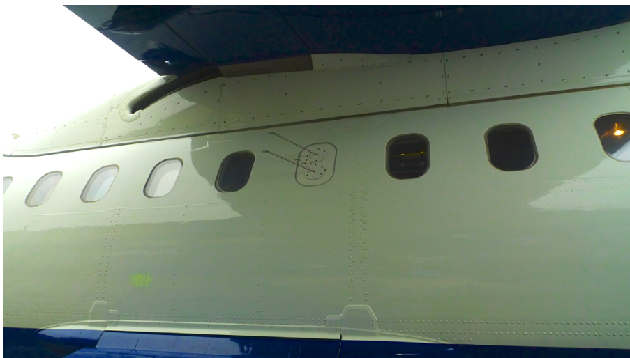
Fig. 2a. Outboard view of the FAAM core chemistry instrumentation inlet window fitted on starboard side window #14, under the BAe 146 wing. The lower 3/8" OD rearward facing SS tube is the FGGA dedicated inlet. The short 1/4" OD rearward facing SS tube is the calibrant outboard vent.
