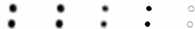
(a) Original images (b) Filtered images (c) Restored images (d) Binary images (e) Particles contour
