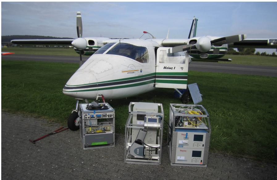
**Fig. 3.** Instruments, mounted in racks, for ready installation in the Partenavia P68B airplane behind. The particle inlet can be seen on top of the fuselage (picture taken by B. Schneider, enviscope GmbH).
