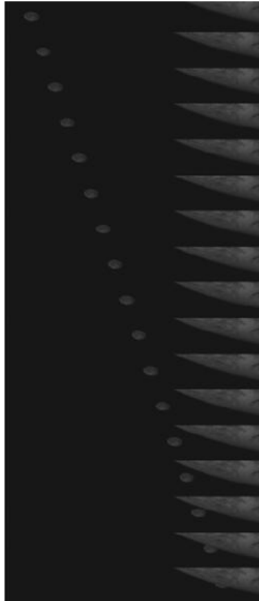
Fig. 3. Series of images taken for the lunar observation on 28 July for the test of the scan mechanism and accuracy of the coordinate system.
