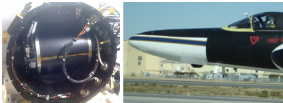
Fig. 1. Left: Pressure vessel and cylindrical drum housing the AirMSPI camera. Right: AirMSPI installed in the nose of the ER-2. The instrument is visible protruding below the fuselage.
