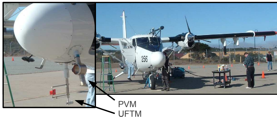
Fig. 2. UFT-M and other fast-response sensors mounted close together around a nose of the Twin Otter Research Aircraft during POST.
