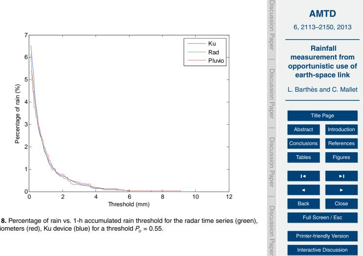
Fig. 8. Percentage of rain vs. 1-h accumulated rain threshold for the radar time series (green), pluviometers (red), Ku device (blue) for a threshold  $P_o = 0.55$ .
