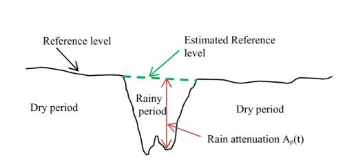
Fig. 6. Received signal during a rain event.
