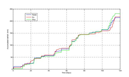
**Fig. 10.** Accumulated rainfall obtained by radar (blue curve), Pluviometer (green curve), attenuation measurements (red curve) during 4 months.
