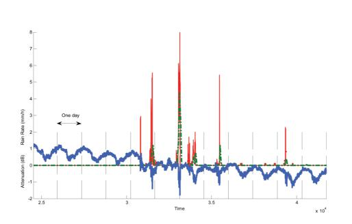
**Fig. 5.** Example of obtained time series: received signal (blue curve), radar rain rate (red curve), 1-h accumulated rainfall time series (dash green curve).
