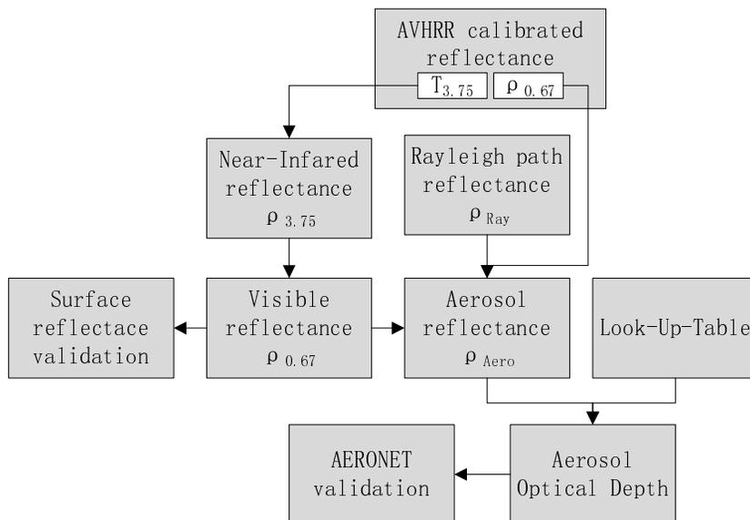
**Fig. 3.** Scheme of the main steps of AVHRR retrieval procedure.
