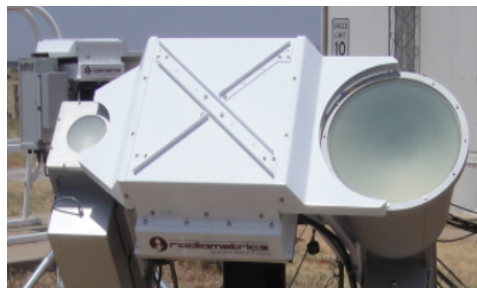
Fig. 5. The new ARM 3-channel microwave radiometer (MWR3C) with a view of the rain mitigation system.
