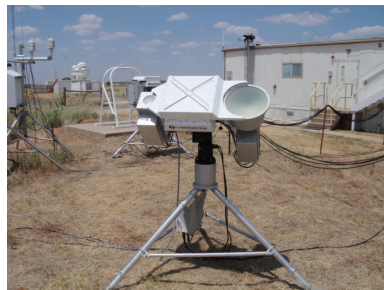
Fig. 5. The new ARM 3-channel microwave radiometer (MWR3C) with a view of the rain mitigation system.
