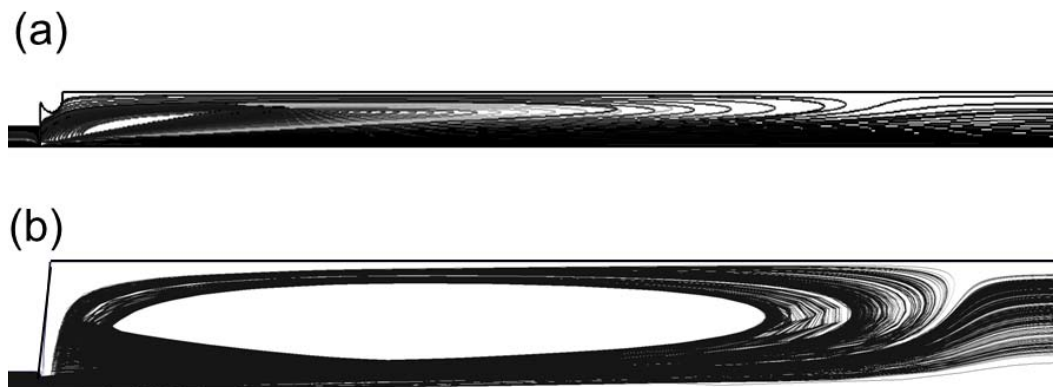
Fig. 2. Calculated trajectories for 3 \mu\text{m} diameter particles (a) without and (b) with relaxation chamber.
