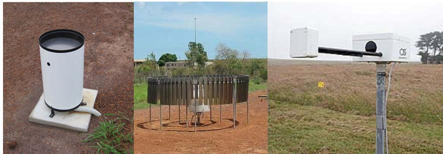
(a) Tipping bucket rain gauge (b) Weighing bucket rain gauge
